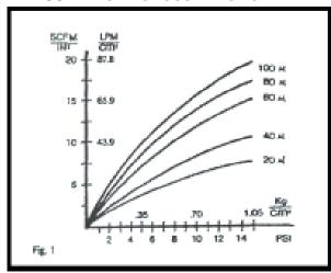
Example: Determine pressure drop through 1/8" thick 40 micron material at a flow of 3 GPM/IM². Use Figure 1 and read down left side to 3, then across to the 40 micron curve, and down to 30 PSI. To determine the pressure drop for 3/8" material under the same flow conditions, use the following equation:
