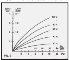
Example: Determine pressure drop through 1/8" thick 40 micron material at a flow of 3 GPM/IM<sup>2</sup>. Use Figure 1 and read down left side to 3, then across to the 40 micron curve, and down to 30 PSI. To determine the pressure drop for 3/8" material under the same flow conditions, use the following equation:
